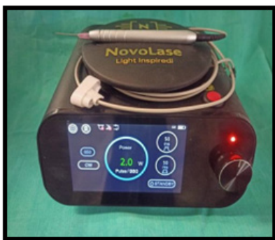
Figure 1: Diode laser: 980 wavelength, power-2 watt, continuous wave.
